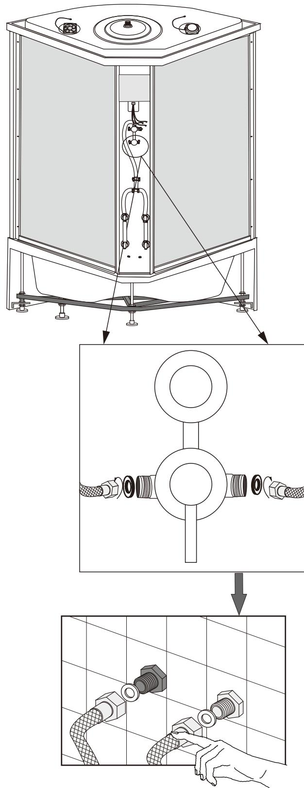
The hot and cold water pipe and connect parts should be bought by client.
