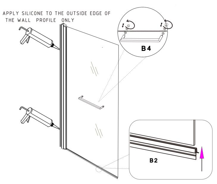
FIX THE BOTTOM SEAL TO THE PIVOT GLASS PANEL
